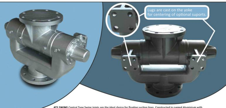
ATS SWING Central Type Swing Joints are the ideal choice for floating suction lines. Constructed in rugged Aluminium with Stainless Steel bearings. ATS SWING Aluminium swing joints are Internally & Externally epoxy painted for Jet-A1 service ATS SWING Joints are available in 8" through 36" size. Larger sizes are available on application. All flanges are ANSI 150# Flat Face or Raised Face.
